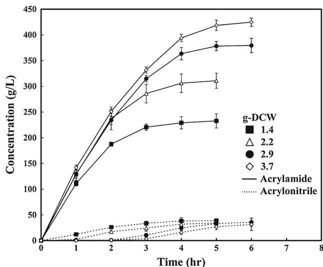
**Fig. 5** Conversion profile of acrylonitrile into acrylamide by recombinant *Corynebacterium* cells. The conversion was carried out in a 2-L jacketed stirred reactor at 18 °C for 6 h. The acrylonitrile solution was continuously fed into the reactor. Experiments were carried out in duplicate, and averages and error bars are presented
