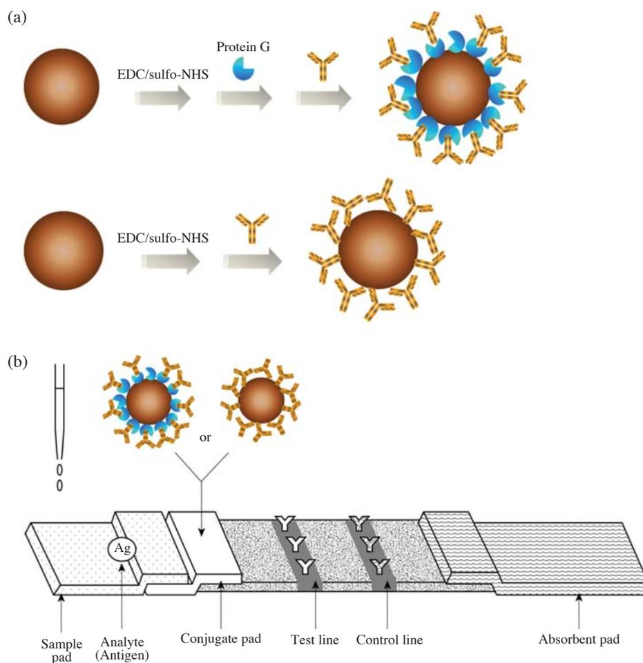
**Scheme 1.** Schematic representation for the lateral flow assays using magnetic labels. (a) Immobilization of antibodies onto magnetic beads in oriented and random manners. (b) Lateral flow assay of a target analyte using magnetic labels.
