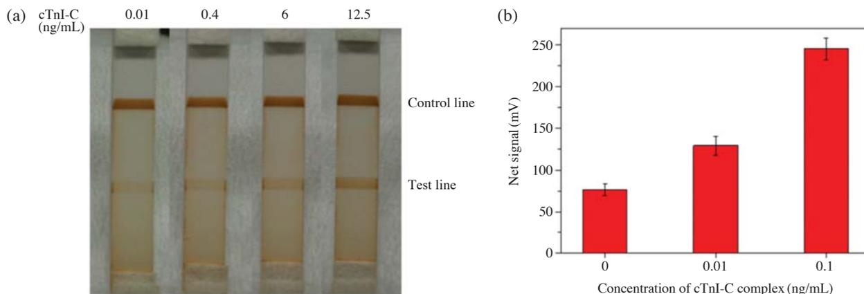
**Figure 2.** Correlation between the concentration of cTnI-C complex and signal intensity in the lateral flow assays (a). The concentrations of cTnI-C complex tested were 0.01, 0.4, 6, and 12.5 ng/mL. The signals in the test line by a GMR sensor when the concentrations of cTnI-C complex were 0, 0.01, and 0.1 ng/mL (b). Bars indicate standard deviations ( $n=5$ ).
