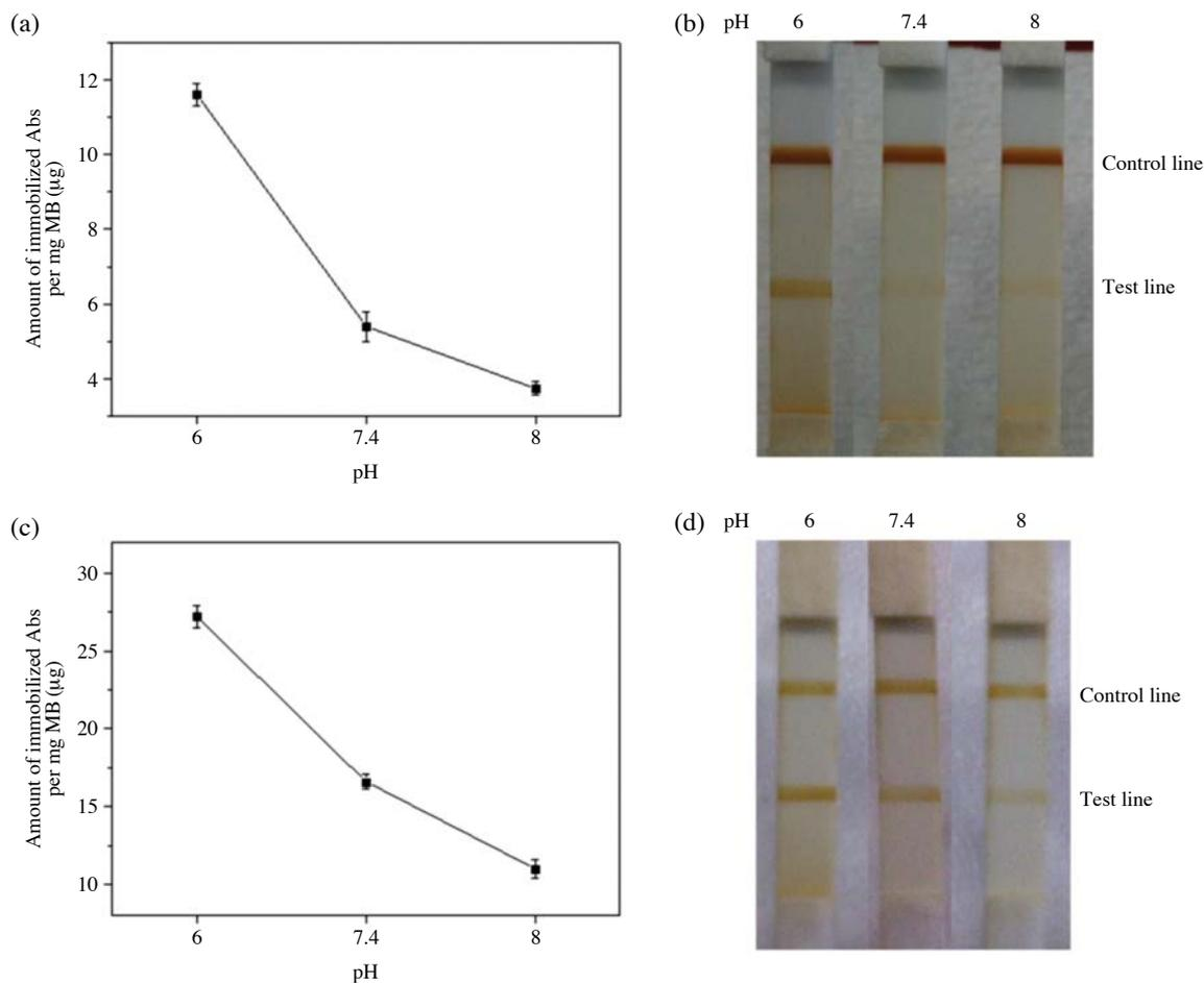
**Figure 1.** Effects of pH on the amounts of immobilized antibodies and signal intensities in the test lines when antibodies were immobilized by oriented approach (a, b) and random covalent conjugation method (c, d). The concentration of cTnI-C complex used for the assays was 25 ng/mL.
