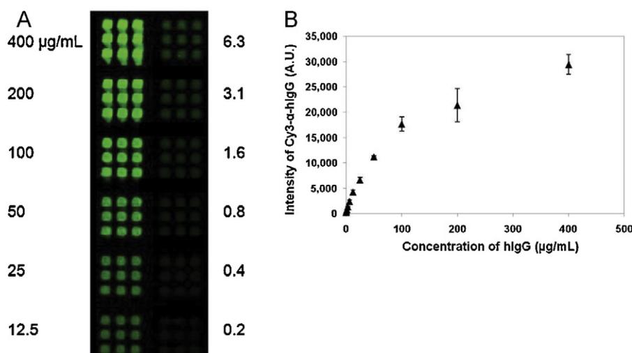
**Fig. 2.** Fluorescence image and intensity of purified hlgG spots. The levels of hlgG were probed by Cy3- $\alpha$ -hlgG, followed by scanning with a fluorescence scanner. The hlgG was serially diluted and spotted on the glass slide in nine spots with a  $3 \times 3$  format using a robotic microarrayer, followed by probing with Cy3- $\alpha$ -hlgG. (a) Fluorescence image of the spots. (b) Changes in the fluorescence intensities of the spots.
