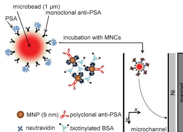
**Scheme 1.** Magnetophoretic assay system using MNCs. PSA is captured by anti-PSA antibody on a microbead, and the resulting microbead is incubated with MNCs for magnetic labeling. The MNC-associated microbead is subjected to injection into a microfluidic channel under a magnetic-field gradient, and its deflection velocity toward the  $x$  axis is determined.
