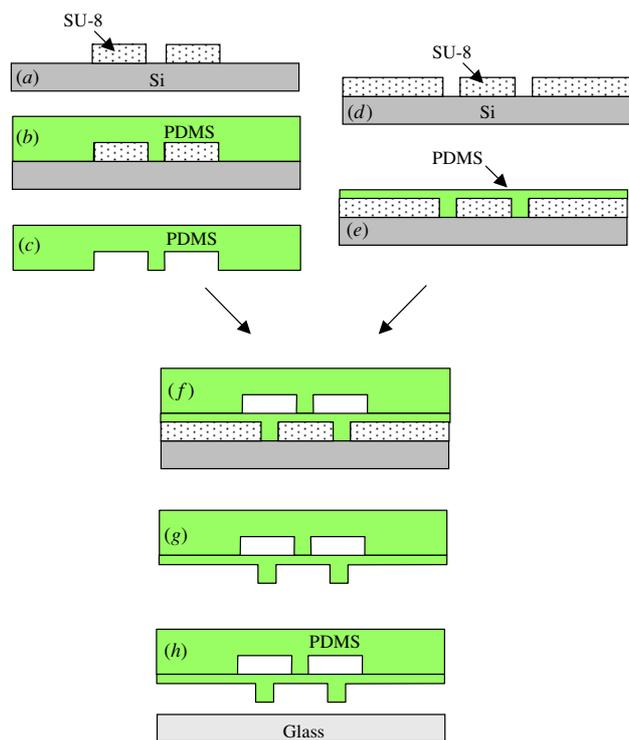
**Figure 2.** Fabrication processes. (a) SU-8 mould patterning for the top PDMS plate, (b) PDMS pouring and curing, (c) PDMS peeled off from the mould, (d) SU-8 mould patterning for the bottom PDMS membrane, (e) PDMS spin coating and curing, (f) bonding the top and bottom PDMS plates, (g) peeling off of the bonded PDMS layer from the substrate and (h) bonding with the glass substrate.
