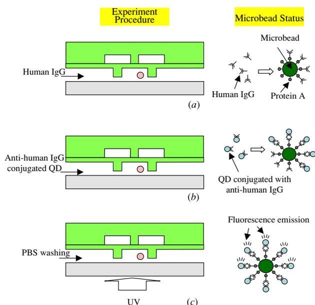
**Figure 4.** The experimental procedures. (a) Human IgG injection after bead capturing, (b) introduction of anti-human IgG conjugated with QD after washing and (c) washing with PBS and fluorescence detection.
