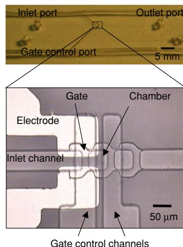
**Figure 3.** Photograph of the fabricated microfluidic chip and a magnified view of a micro-chamber.
