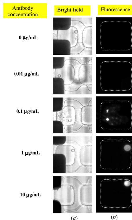
**Figure 5.** Experimental results. (a) Bright field (not fluorescence) images of each micro-chamber with the captured single microbead and (b) fluorescence images for various concentrations of antibodies in a corresponding micro-chamber.
