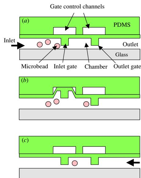
**Figure 1.** Schematic view of each step for the capturing of a single microbead. (a) Bead introduction, (b) gate open and (c) gate closed/single bead captured.
