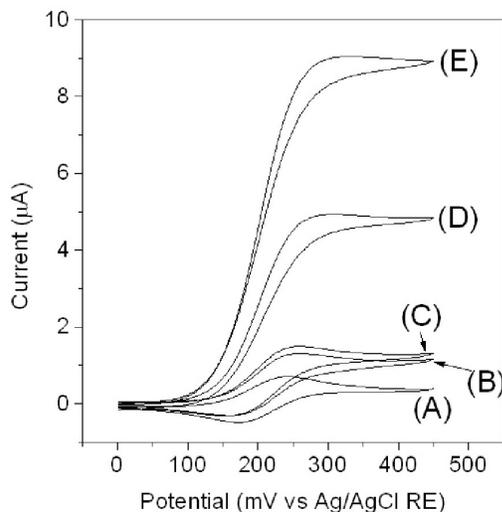
**Fig. 3.** Cyclic voltammograms of affinity biosensors for avidin by the signaling mode of the diffusible mediator-facilitated electron transfer: (A) background, (B) 0 µg/mL avidin, (C) 100 µg/mL, (D) 1 mg/mL, and (E) 2 mg/mL. Conditions for the electrochemical tests were the same as Fig. 2.
