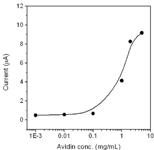
**Fig. 4.** The calibration curve from the resulting affinity biosensors for avidin by the signaling mode of the diffusible mediator-facilitated electron transfer.
