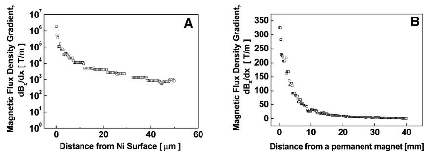
**Figure 2.** Comparison of the simulated results between a permanent magnet and a Ni microstructure under external magnetic field: profiles of simulated magnetic field gradient (A) with a Ni microstructure under external magnetic field and (B) with a permanent magnet only.
