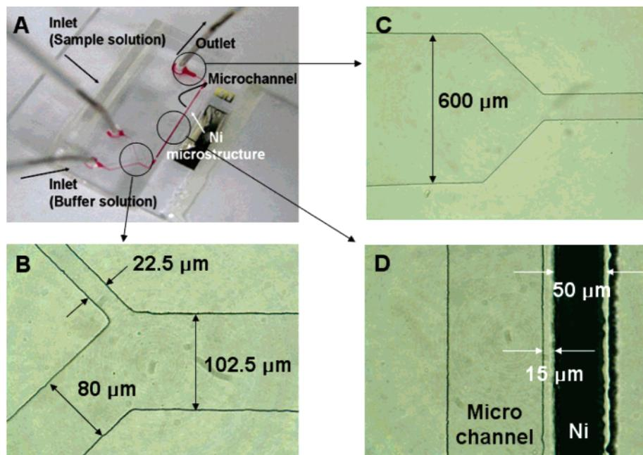
**Figure 1.** (A) Photograph of the microfluidic device with a Ni microstructure and optical microscope images of the microchannels; (B) inlet part, (C) outlet part (expansion part), and (D) microchannel that is 15  $\mu\text{m}$  apart from the Ni microstructure.
