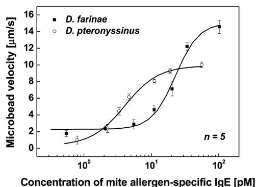
**Figure 4.** Deflection velocities of microbeads with respect to the concentrations of *D. farinae* and *D. pteronyssinus* allergen-specific human IgEs, respectively. The velocities of five microbeads were independently determined. Error bars indicate the means and standard deviations of measurements.
