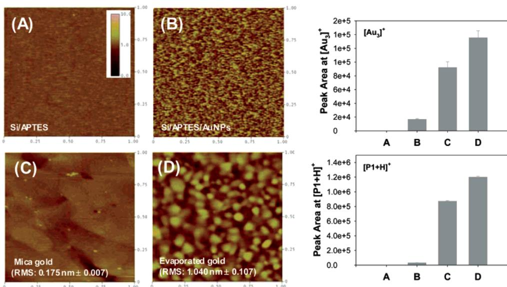
**Figure 5.** Comparison of ion peak areas ( $[Au_3]^+$  and  $[P1+H]^+$ ) on various surfaces. (A) Si/APTES; (B) Si/APTES/AuNPs; (C) mica gold; (D) evaporated gold substrate. The peptide signal was measured after a 60-min period of adsorption onto different surfaces.
