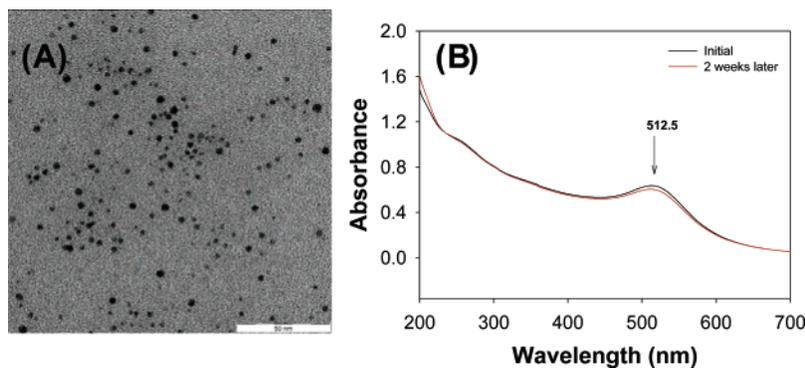
**Figure 1.** (A) Energy-filtering TEM image and (B) UV–visible spectrum of citrate-stabilized AuNPs. Mean diameter of AuNPs is 3.2 nm (SD  $\pm 0.4$ ,  $n = 100$ ). The UV spectrum of AuNPs in solution was stable for 2 weeks.
