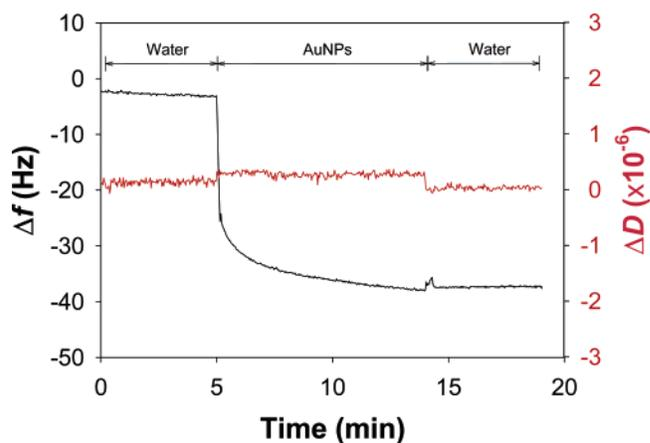
**Figure 3.** QCM response of AuNPs and peptides sequentially adsorbed on to amine-terminated MUAM SAMs on a gold sensor. Changes in frequency (black line) and dissipation (red line) were simultaneously traced in a 5-MHz crystal.
