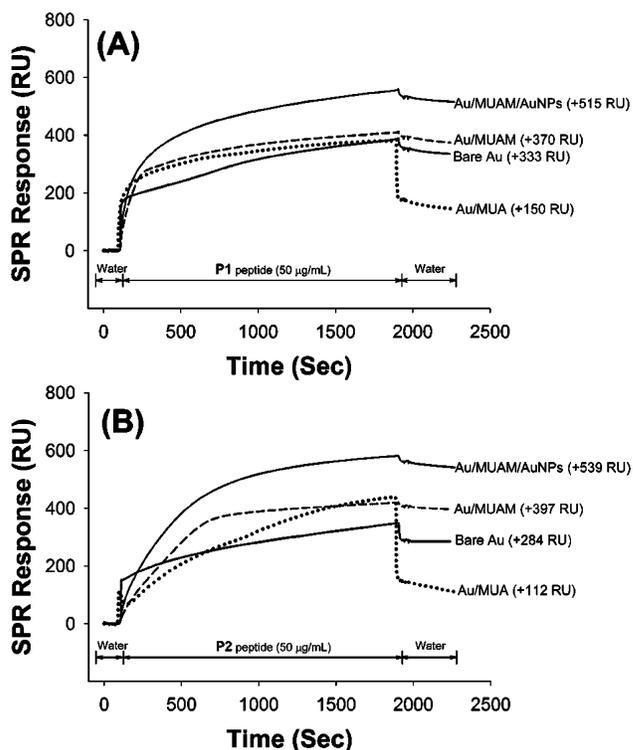
**Figure 6.** Real-time SPR responses of two peptides (P1 and P2) attached to bare Au, Au/MUA, Au/MUAM, and Au/MUAM/AuNPs. (A) P1 and (B) P2 peptides with a solution of  $50 \mu\text{g}\cdot\text{mL}^{-1}$  in distilled water were independently loaded in flow channel 1 and flow channel 2, respectively.
