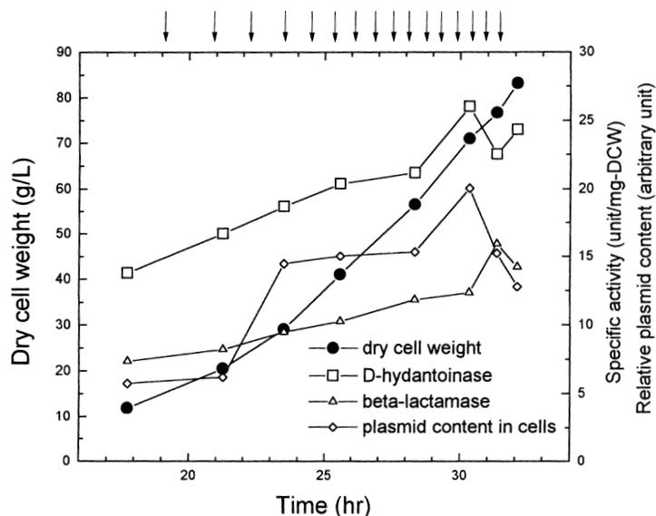
**FIGURE 1.** Fed-batch cultivation of *E. coli* XL1-Blue/pHU183 using glucose as a carbon source at 30 °C. Glucose and  $\text{MgSO}_4$  were fed based on the pH-stat method, and the substrate feedings are indicated by arrows. The fed-batch culture was conducted in duplicate, and the data represent mean values.
