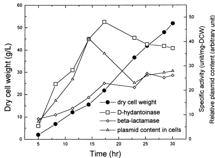
**FIGURE 2.** Batch cultivation of *E. coli* XL1-Blue/pHU183 using glycerol as a carbon source at 37 °C. Cultivations were carried out in a 50-L fermentor containing 35 L of the R-medium. The batch cultivation was carried out in duplicate, and the data represent mean values.
