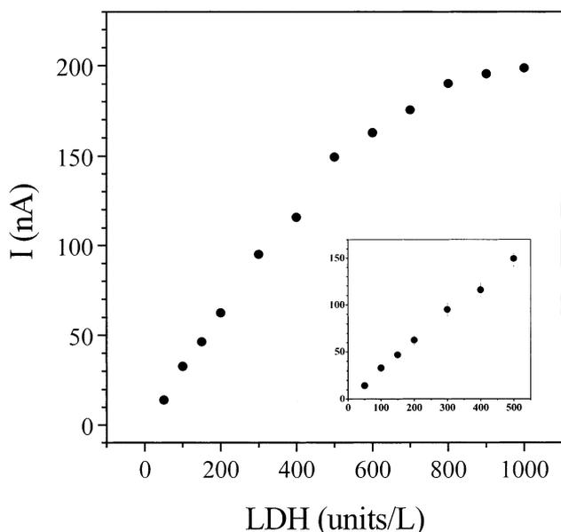
Fig. 6. Calibration curve of the LDH biosensor. The inset indicates calibration curve obtained for the linear range. Steady-state electrocatalytic responses were registered at applied potential of +300 mV vs. Ag/AgCl.
