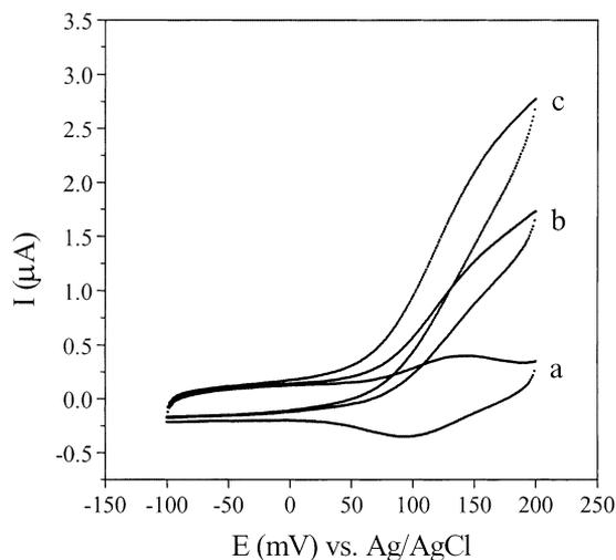
Fig. 3. Electrochemical oxidation of NADH at the 3,4-DHB modified electrode in the absence of NADH (a); in the presence of 0.5 mM NADH (b) and 1 mM NADH (c). Potential scan rate was 10 mV/s.
