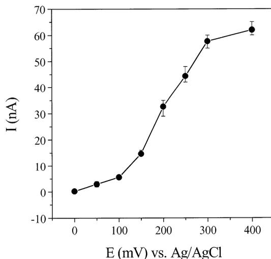
Fig. 5. The amperometric response of the thick-film biosensor to the LDH concentration of 200 U/l as a function of the applied potential.
