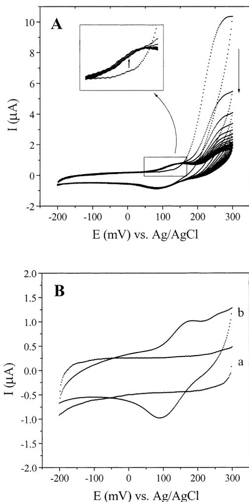
Fig. 1. (A) Electrodeposition process of 3,4-DHB by potential cycling between  $-200$  and  $+300$  mV at  $20$  mV/s. (B) Cyclic voltammogram of the working electrode before (a) and after electrodeposition of 3,4-DHB (b). Potential scan rate was  $5$  mV/s. Electrodeposition and electrochemical measurements were performed in  $0.1$  M phosphate buffer (pH  $8.2$ ).
