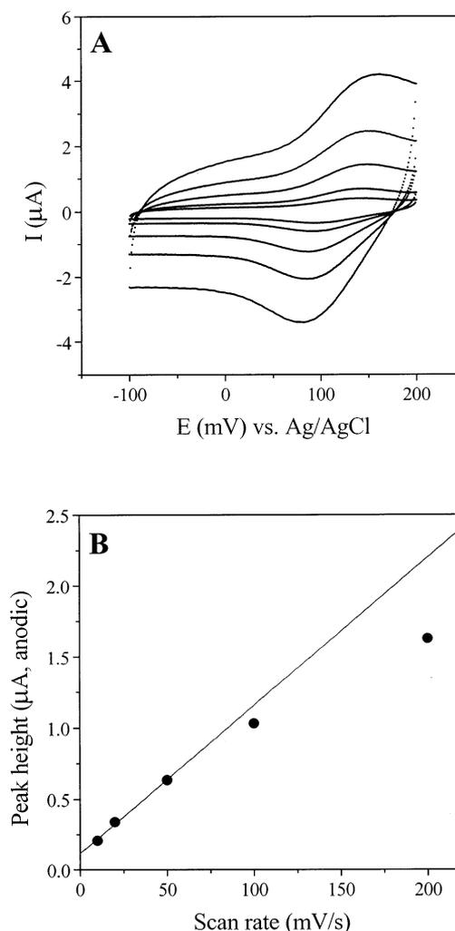
Fig. 2. (A) Cyclic voltammograms of the 3,4-DHB modified electrode at different potential scan rates:  $10$ ,  $20$ ,  $50$ ,  $100$  and  $200$  mV/s (from inside voltammograms) in  $0.1$  M phosphate buffer (pH  $8.2$ ). (B) Dependence of the anodic peak currents on the potential sweep rate.
