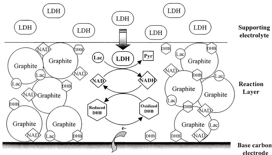
Scheme 1. Reaction scheme of the thick-film LDH biosensor. Abbreviations used: LDH, L-lactate dehydrogenase; Lac, L-lactate; Pyr, pyruvate; NAD,  $\beta$ -nicotinamide adenine dinucleotide; NADH,  $\beta$ -nicotinamide adenine dinucleotide, reduced form; DHB, 3,4-dihydroxybenzaldehyde.
