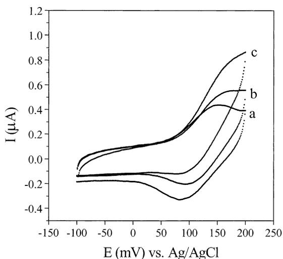
Fig. 4. Electrocatalytic oxidation of enzymatically generated NADH at the working electrode in the absence of LDH (a); in the presence of 0.2 mg/ml LDH (b) and 0.4 mg/ml of LDH (c). Potential scan rate was 10 mV/s.
