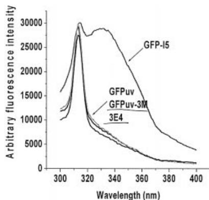
**Fig. 5.** Tryptophan emission spectra of GFP variants (GFP-I5, GFPuv, GFPuv-3M and 3E4). The proteins were excited at 283 nm and the fluorescence was scanned at 300–400 nm. The fluorescence intensity is in arbitrary units.
