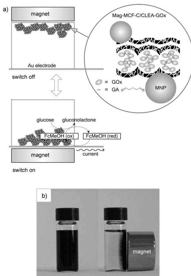
**Figure 1.** a) Working principle of the magnetically switchable bio-electrocatalytic oxidation of glucose by GOx immobilized in Mag-MCF-C. b) The separation of Mag-MCF-C/CLEA-GOx particles by an applied magnetic field. The image shows a well-mixed suspension of Mag-MCF-C/CLEA-GOx in 0.1 M sodium phosphate buffer (ca.  $10 \text{ mg mL}^{-1}$ ) before (left) and after (right) the application of a magnetic field.
