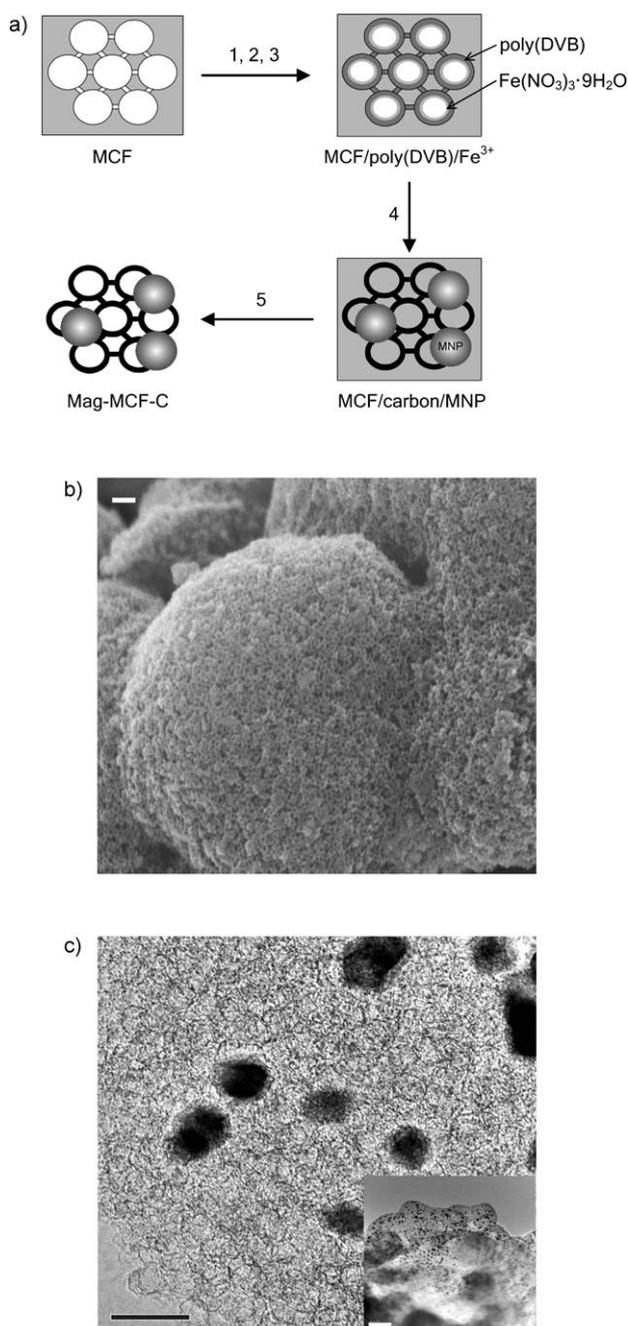
**Figure 2.** a) Schematic representation of the synthetic procedure for Mag-MCF-C: impregnation of DVB/AIBN (1); polymerization (2); impregnation of  $\text{Fe}(\text{NO}_3)_3 \cdot 9\text{H}_2\text{O}$  (3); carbonization (4); removal of silica template (5). b) SEM image of Mag-MCF-C (scale bar: 200 nm). c) TEM image of Mag-MCF-C (scale bar: 50 nm); inset: low-magnification TEM image of Mag-MCF-C (scale bar: 500 nm). AIBN = azobisisobutyronitrile.
