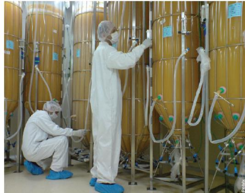
Protalix's bioreactor plant cell system. The GMP-approved system is set up to manufacture a range of proteins, including antibodies, complex enzymes and plant-derived pharmaceuticals.
